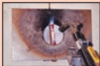
Fire test of protective sleeveings
